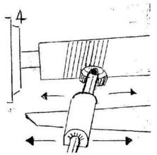
4. Turn the lathe back on and with the tool flat, gently present the cutter back on to the wood and again gently raise the handle to allow the cutting wheel to follow the grooves you made in step 2. Then move the tool along the wood to the length of the Spiral required, cutting deeper on each pass. Repeat this until the required depth of your Spiral has been cut.
