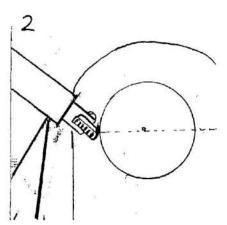
2. Gently place the cutter against the wood, then raise the handle as the cutter spins, cutting on the centre line of your turning.
